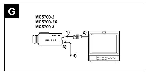
Connecting the Monitor to the MC5700 Series Cameras (Illustration A)
